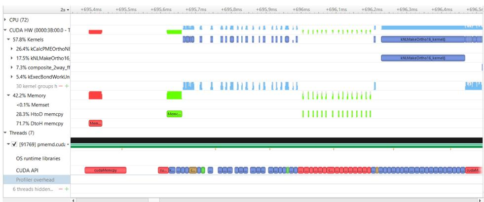
**Figure 4.** Results of profiling the Plumed-enabled pmemd.cuda\_SPFP executable version (CUDA 11.1) with NVIDIA Nsight Systems. 1 ms is shown. Data exchange between CPU and GPU takes about 42% of all calculation time while “computational kernels” execution takes about 58% of time
