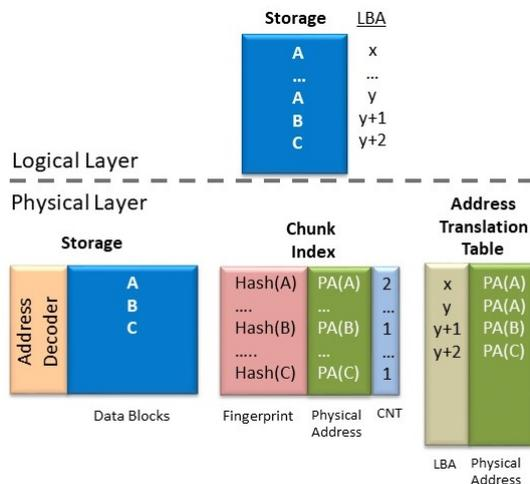
**Figure 5.** Conventional deduplication scheme after writing the following sequence of (data block, LBA): (A, x), (A, y), (B, y+1), (C, y+2). The storage, chunk index and address translation table reside in the physical layer
